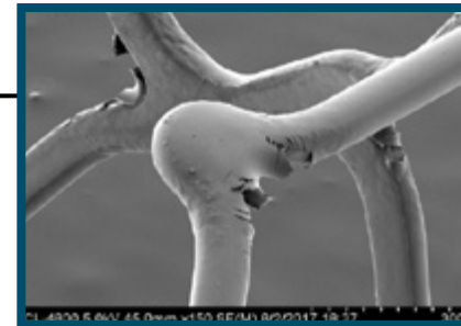
SYNERGY (3.5 x 20 mm) 150x magnification at max expansion of 4.25 mm
